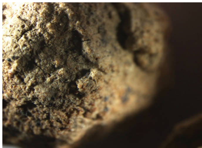
Figure 4: LDA size (4-8) mm (Plate 1): Sintered fly ash aggregate. Nodule with corroded surface and open voids grains in agglomerated form (1.5x)
