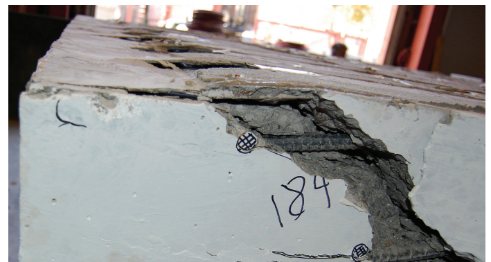
Figure 8: Damage at ultimate capacity showing concrete cracking and local debonding of the NSM FRP adhesive from the concrete in the right figure
