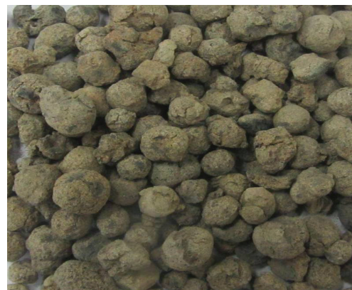
Figure 3: External appearance of sintered fly ash aggregate or LDA (30x)
