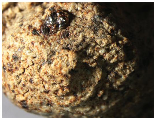
Figure 5: LDA size (4-8) mm (Plate 2): Sintered fly ash aggregate. Nodule with smooth surface and cluster of sintered material (1.5x)
