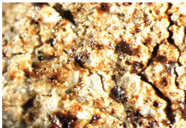
Figure 6: LDA size (8-16) mm (Plate 1): Sintered fly ash aggregate. Nodule with smooth surface and cluster of sintered material (2.5x)
