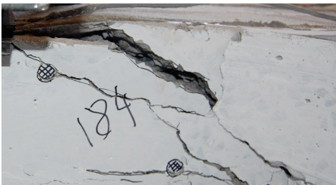
Figure 8: Damage at ultimate capacity showing concrete cracking and local debonding of the NSM FRP adhesive from the concrete in the right figure
