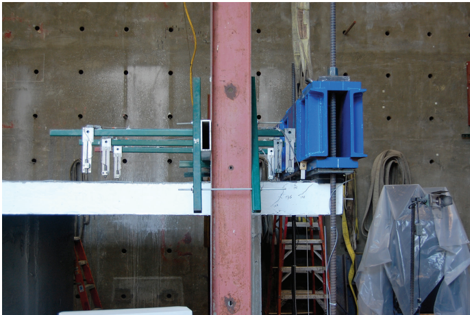
Figure 4(c): Front view of test specimen showing the loading beam and linear potentiometers
